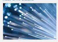
is used for optical data transmission. Compared with traditional means via copper cable, it offers a far higher maximum bandwidth. Optical fibers are also insensitive to electrical and magnetic interference fields and offer higher immunity to tapping.
